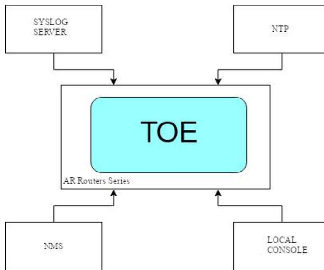
**Figure 1-1** IT Entities which connect with TOE
