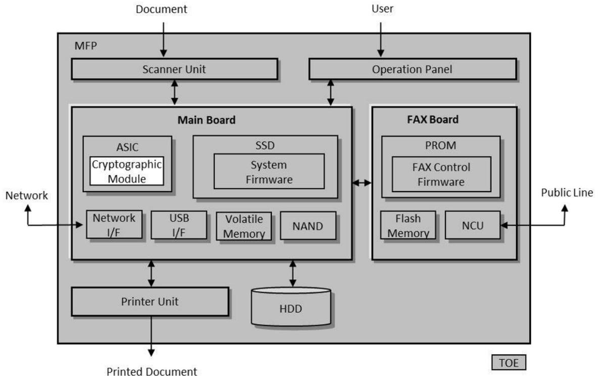
The TOE consists of an Operation Panel, a Scanner Unit, a Printer Unit, a Main Board, a FAX Board, HDD and SSD hardware, and firmwares.
