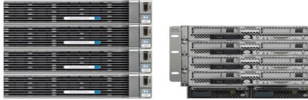
**Figure 5 Cisco HyperFlex HX240c M4 Nodes with Cisco UCS B200 Blade Servers**
