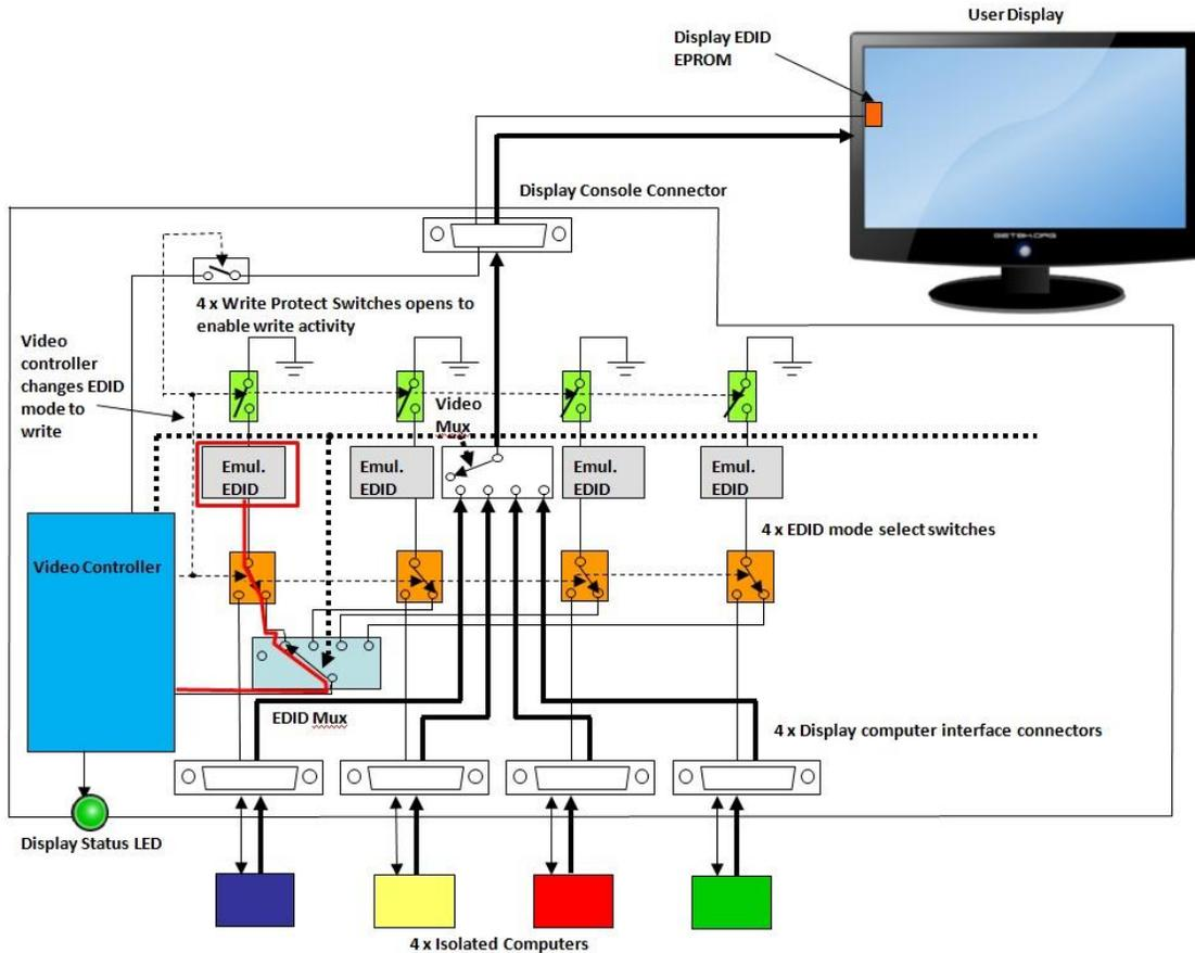
**Figure 15 – Display EDID Write Function**
