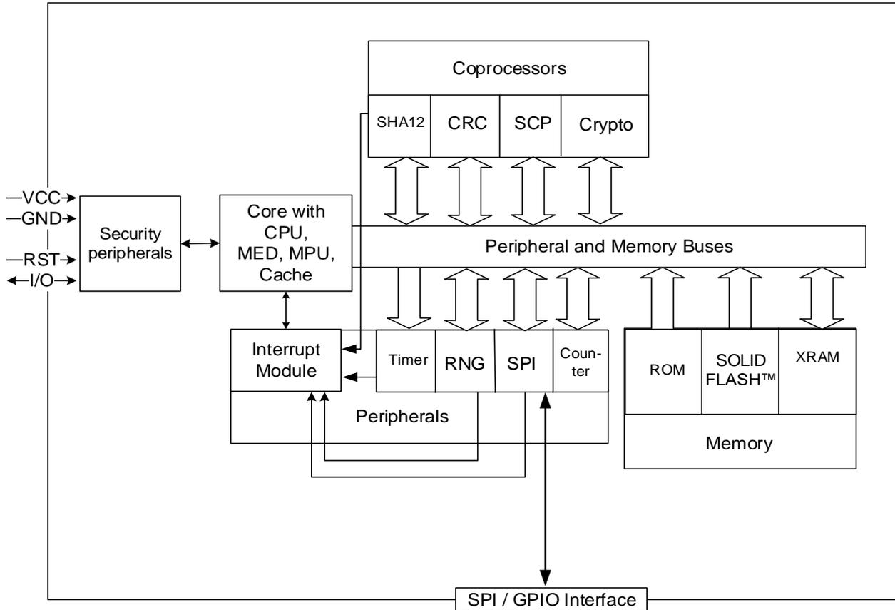
Note: The SLB9672\_2.0 v16 includes an SPI interface, the SLB9673\_2.0 v26 includes an I2C interface.
