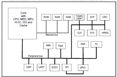
Logically the TOE provides cryptographic support for TDES, AES, and RNG, memory protection unit supporting different memory access levels, authentication of the smartcard IC, support for loading of flash content in secured locations and in loading by authorized users only.
