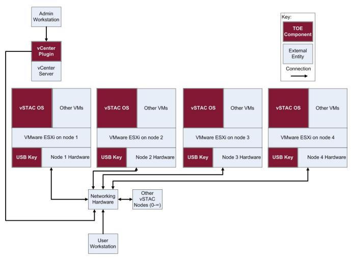
Figure 2 – Deployment Configuration of the TOE
