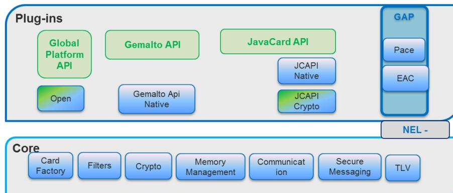
**Figure 2: MultiApp V5.0.A Java Card platform architecture**
