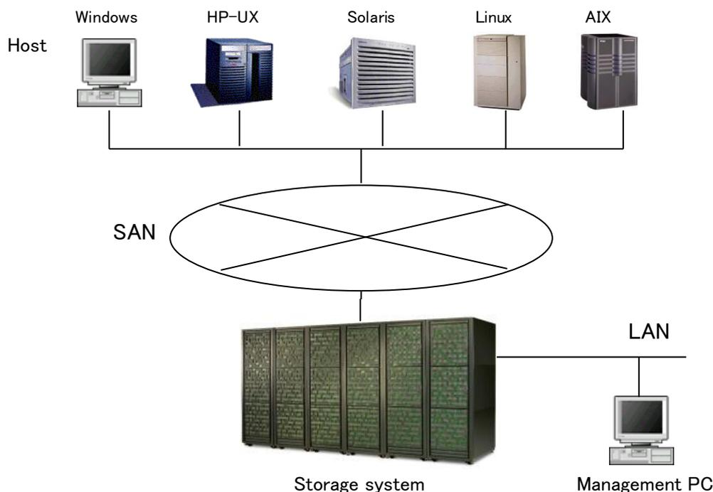
**Figure 1-1 General system configuration including storage system**
