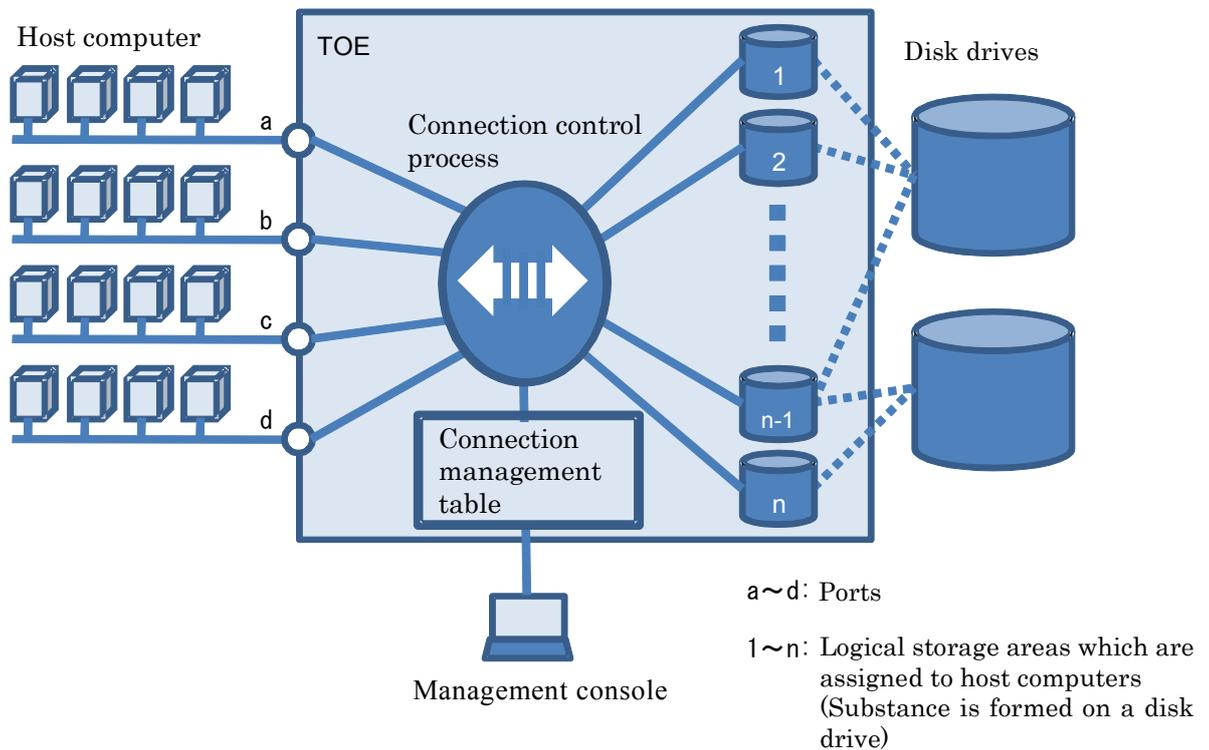
Figure 1-3 Connection control between host computers and logical storage areas
