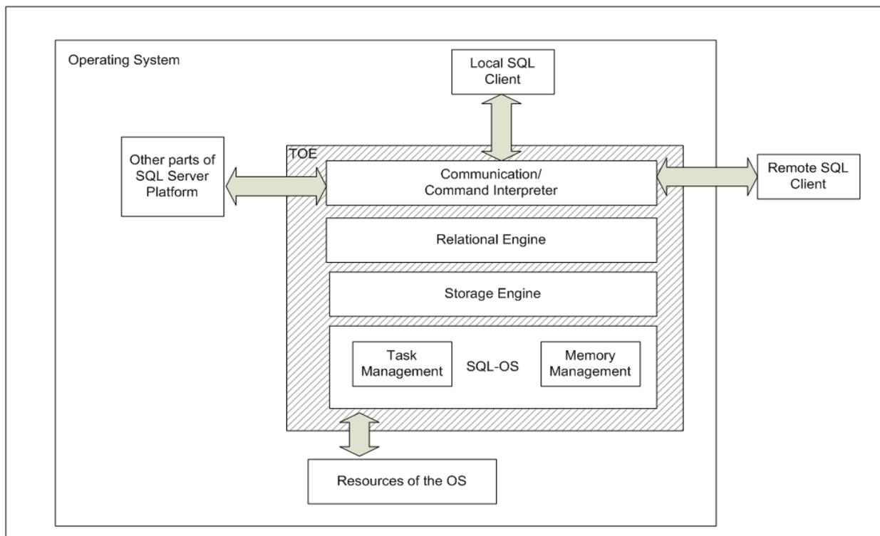
**Figure 1 - TOE Structure**
