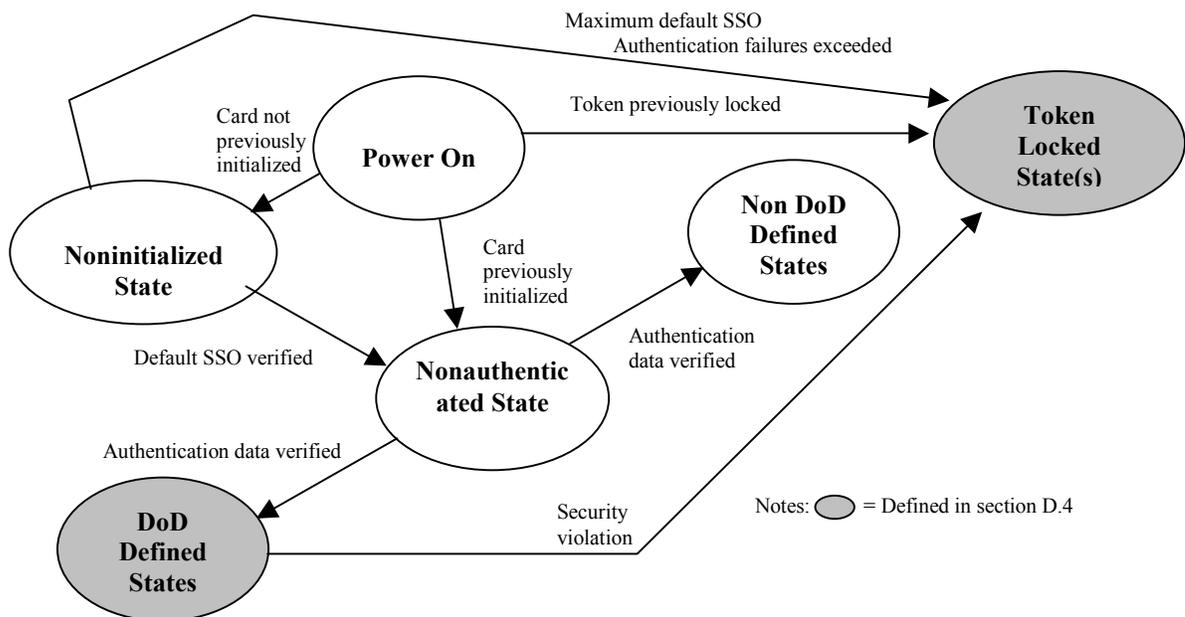
**Figure D-1 Token Top Level State Diagram**
