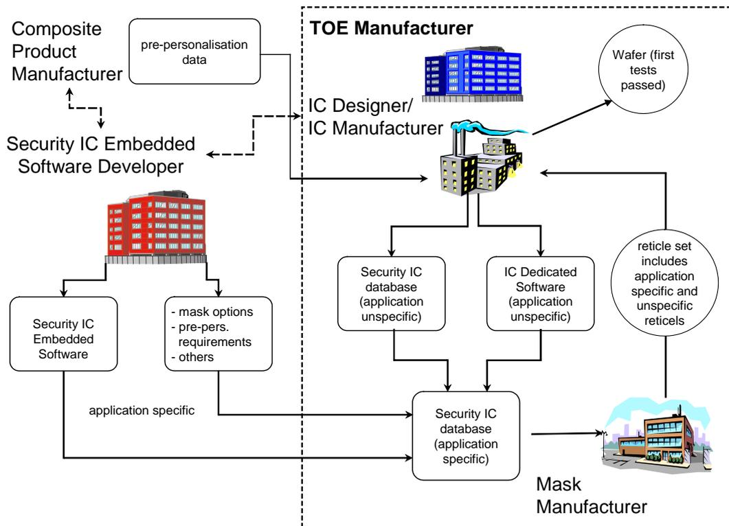
Figure 18: Development and Wafer Production including Testing in case of Embedded Software in ROM and EEPROM only
