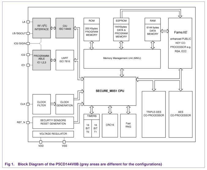
There are differences in the configurations, indicated in grey in the figure. Refer to section 2.2 for information about the configurations. The following tables list the TOE
