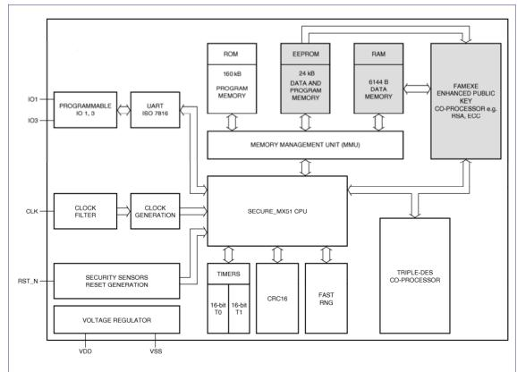
Fig 1. Block Diagram of the P5CC024/ P5CC020/ P5CC012V0A (grey areas are different for the configurations)
