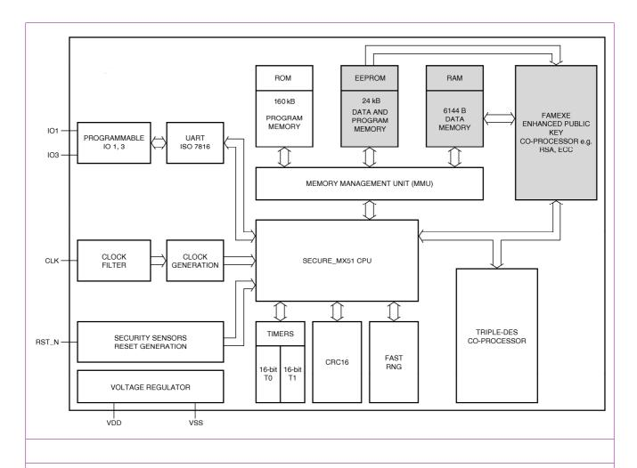
Fig 1. Block Diagram of the P5CC024/P5CC020/P5SC020/P5CC012V0A (grey areas are different for the configurations)
