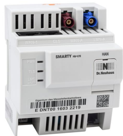
Figure 3: SMARTY IQ-SMGW LTE casing and external interfaces
