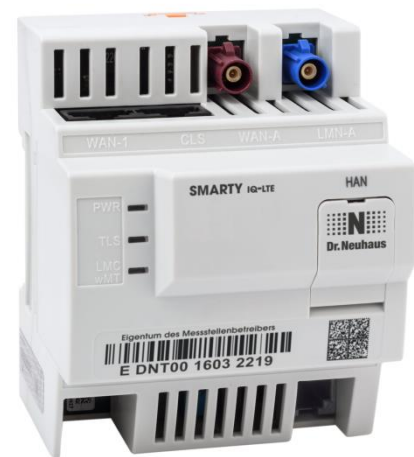
Figure 3: SMARTY IQ-LTE casing and external interfaces
