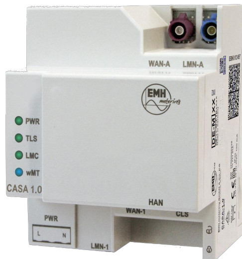
Figure 5: Casing of the TOE with optional HAN module
