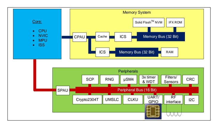
The TOE hardware consists of a core, a memory system and peripherals.
