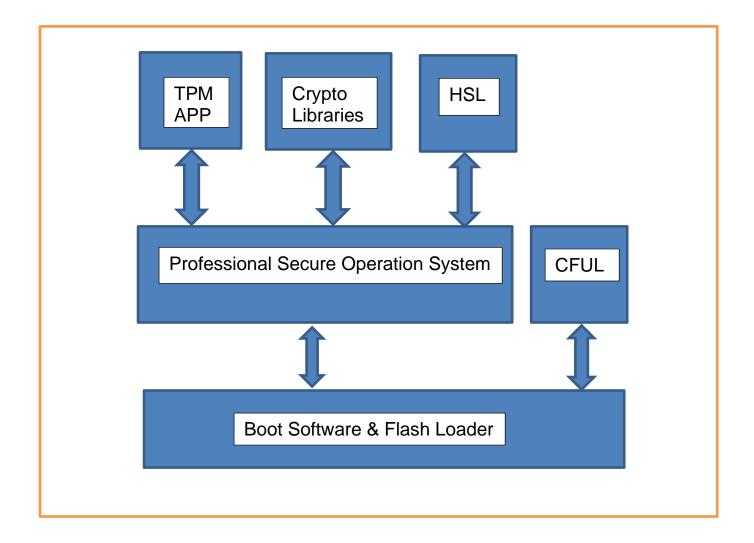
Figure 2: Firmware block diagram of the TPM
