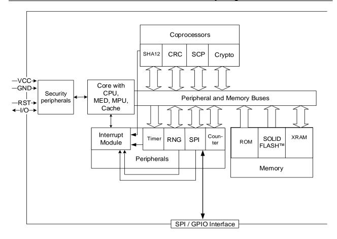
Note: The SLB9672\_2.0 v17 includes an SPI interface, the SLB9673\_2.0 v27 includes an I2C interface.
