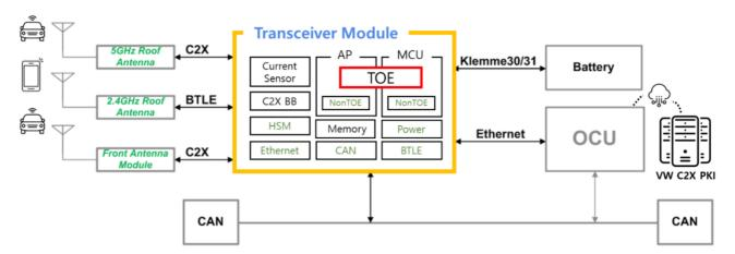
The TOE is used by integrating it into the application processor (AP) and the microcontroller unit (MCU) elements of the transceiver module. The TOE consists of system interface for communication, C2X stack and service layer. Furthermore, they are packaged in one binary file.
