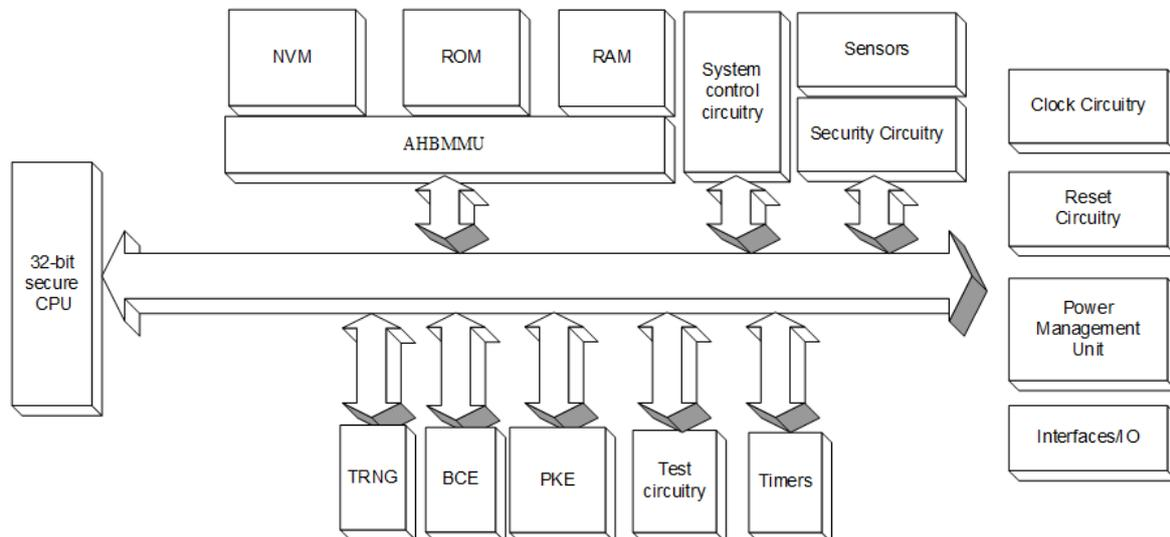
The hardware of the TOE has the following components:
