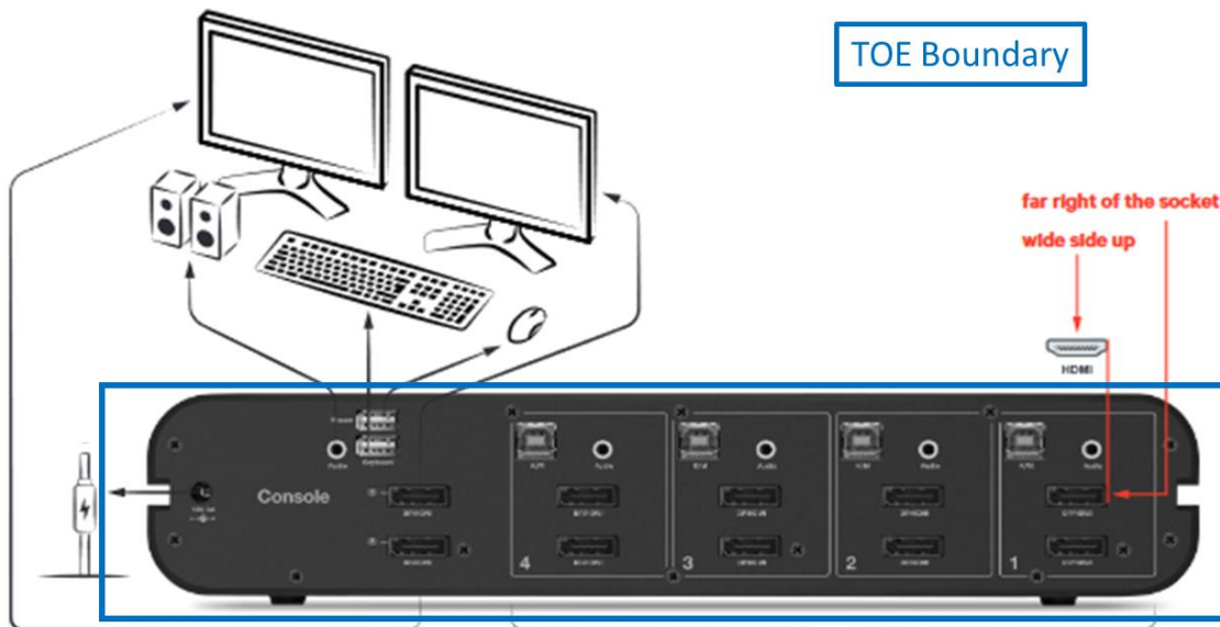
Figure 2 – Typical example of KVM TOE installation
