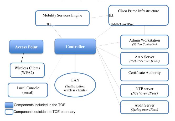
Figure 1: Sample TOE Deployment
