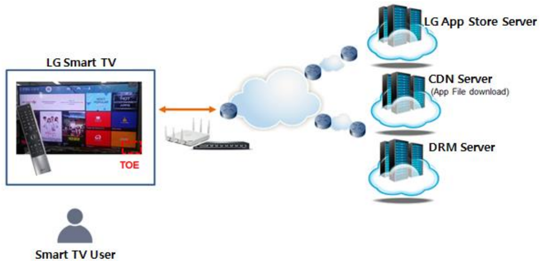
[Figure 1] TOE Operational Environment - IT Entities outside of Smart TV
