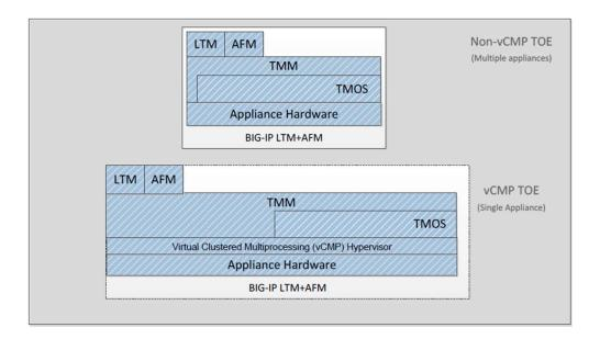
The TOE is separated into two distinct planes, the control plane and the data plane. The control plane validates, stores, and passes configuration data to all necessary systems. It also provides all administrative access to the TOE. The data plane passes user traffic through the TOE.
