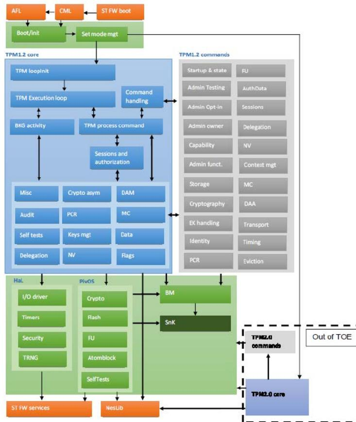
Figure 2 – Architecture *firmware*
