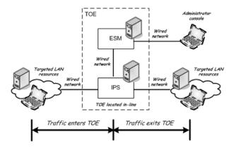
The general concept of operation of the TOE in *an in-tap network location operating in an IDS mode* is depicted in the figure below:
