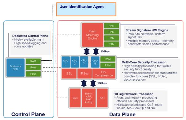
The control plane includes a dual core CPU, with dedicated memory and a hard drive for local log, configuration, and software storage. The data plane includes three components, the network processor, the security processor, and
