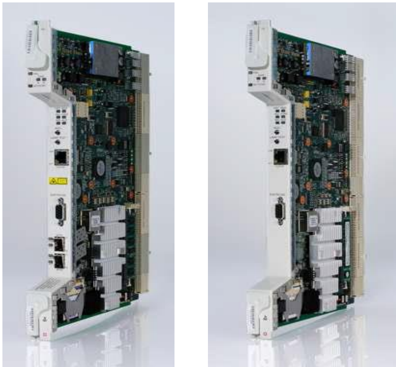
Figure 2 Cisco ONS 15454 TNC Card and ONS 15454 TSC Card
