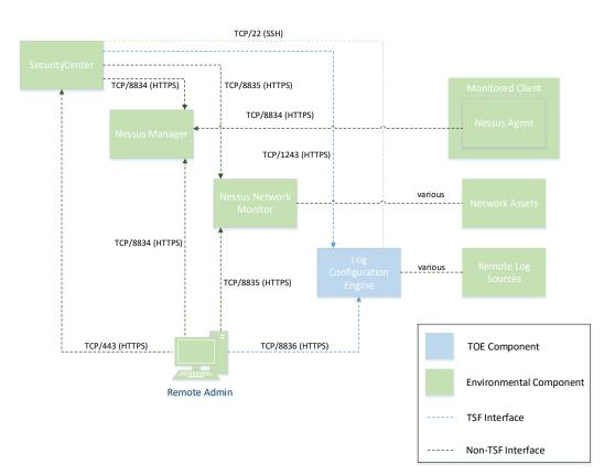
Figure 1 – Example Deployment
