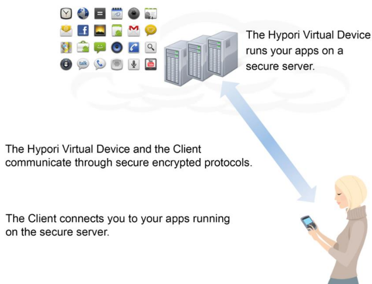
Figure 2 Hypori Client as Part of VMI Platform
