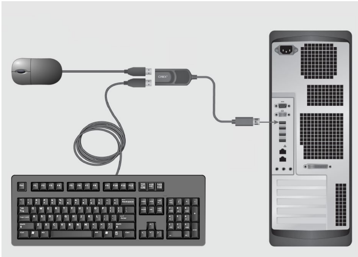
Figure 2 – USB Filter Evaluated Configuration
