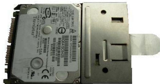
Figure 6. SecureD mounted in desktop adapter – data and power interfaces
