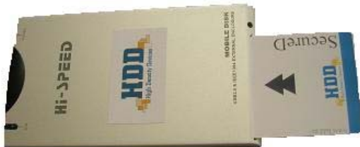
Figure 7. SecureD mounted in an external, USB drive carrier
