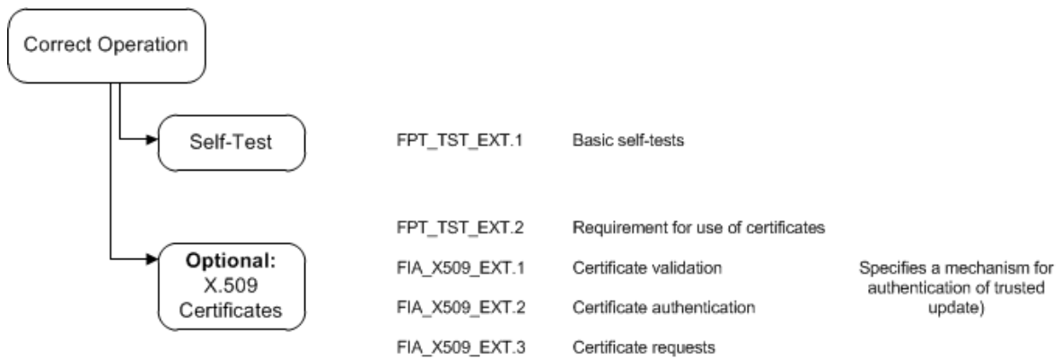
Figure 3: Correct Operation SFR Architecture
