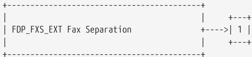
FDP\_FXS\_EXT.1 Fax Separation, requires the fax interface cannot be used to create a network bridge between a PSTN and a LAN to which TOE is connected.
