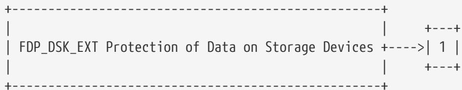
FDP\_DSK\_EXT.1 Protection of Data on Storage Devices, requires the TSF to encrypt all the Confidential TSF and User Data stored on the Nonvolatile Storage Devices in order to avoid storing these data in plaintext on the devices.
