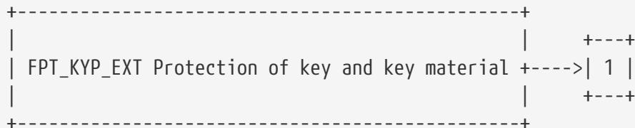
FPT\_KYP\_EXT.1 Protection of key and key material, requires the TSF to ensure that no plaintext key or key materials are written to nonvolatile storage.
