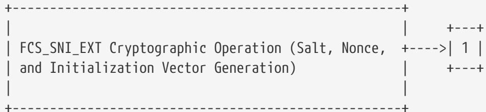
FCS\_SNI\_EXT.1 Cryptographic Operation (Salt, Nonce, and Initialization Vector Generation), requires the generation of salts, nonces, and IVs to be used by the cryptographic components of the TOE to be performed in the specified manner.
