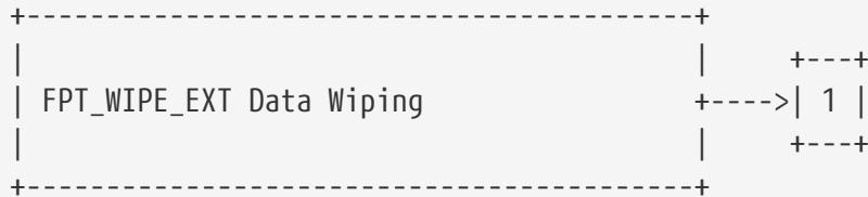
FPT\_WIPE\_EXT.1 Data Wiping, requires the TSF to make User and TSF Data stored on Nonvolatile Storage Devices unavailable upon request of an Administrator using cryptographic erase and optionally additional other media-specific methods.
