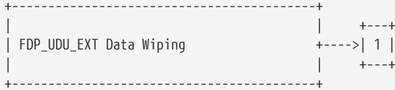
FDP\_UDU\_EXT.1 Document Unavailability, requires the TSF to make User Document Data stored on wear-leveling and non-wear-leveling storage devices unavailable via either overwrite or destruction of cryptographic keys to ensure that this data does not remain on the device in the TOE after a Document Processing job has been completed or cancelled.
