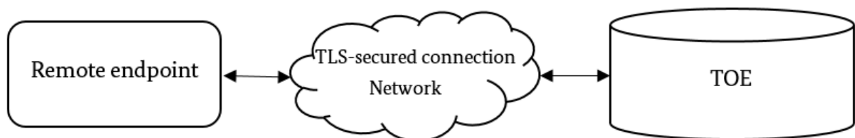
Figure 1: TOE access model
